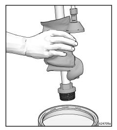
Place fluid intake in flushing fluid. Use water for water-based paint and mineral spirits for oil-based paint. Place drain tube in waste pail.
