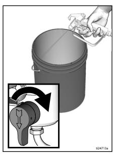
9. Raise fluid intake above flushing fluid.
