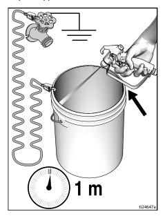
Move gun to paint pail and trigger for 20 seconds. Release trigger and allow sprayer to build pressure. Engage trigger lock.
