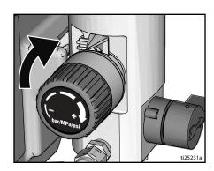
6. Turn prime valve horizontal. Disengage trigger lock.
