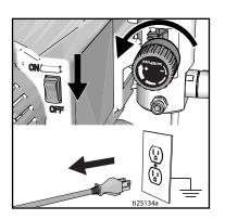
Remove filter from gun and sprayer if installed. Clean and inspect. Install filter. See separate gun manual.
