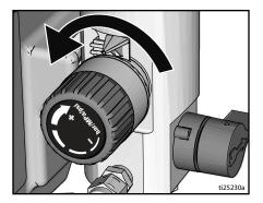
3. Turn ON/OFF switch to ON position.
