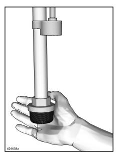
Fill throat packing nut with TSL to prevent premature packing wear. Do this daily or each time you spray.
