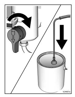
If you suspect the spray tip or hose is clogged or that pressure has not been fully relieved:
