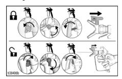
Engage trigger lock. Return Spray Tip to original position. Disengage trigger lock and continue spraying.
