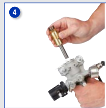
Install new cartridge and replace pump
