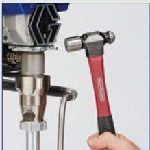
Loosen the clamping nut
