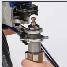
Open door and remove pump
