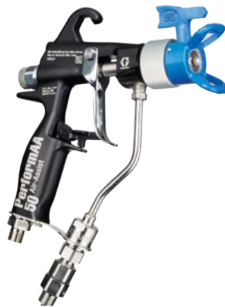
PerformAA 50 RAC ® Air Assist gun sprays with a Reverse-A-Clean ® tip at 345 bar (5,000 psi) for high pressure applications.
