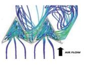
Consequently the static pressure increases only slowly with the accumulation of paint, enabling a uniform airflow around the parts that are being coated, and more importantly clean air environment for the sprayers.
